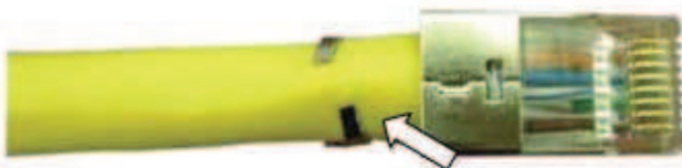
Wrap cable holder around the jacket and tighten with pliers.
