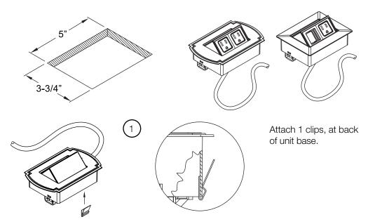
Note: Metal clips are for use in hard surface material only as an optional mounting means
